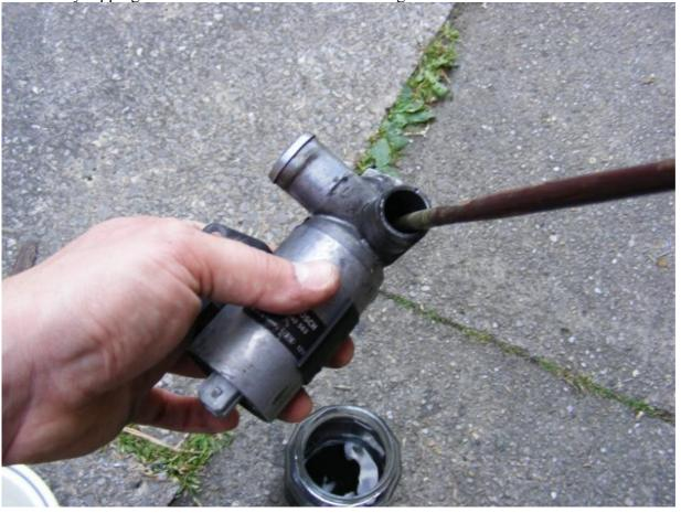
I got bored with that & decided to lay the valve in an old bowl & pour the cleaner directly into it, give it a shake & pour more in then agitate with the brush. I kept filling it & placing the ball of my thumbs over each hole & started to rotate it quickly to get as much of it clean as possible. Repeat this process till it 'sounds' very loose & free:
