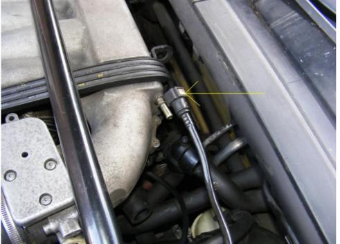
When I removed mine & tried to rotate it, the valve was quite clogged up, it wouldn't rotate all the time, not to mention it sounded extremely blocked. Once it's fully cleaned it will sound very loose inside & very metallic when you rotate it, that's because there's no build up in there anymore.
